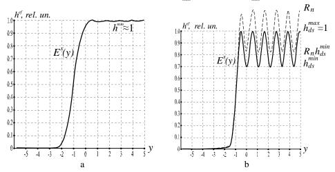
**Fig. 2.** Edge functions in the direction of the frame scan: a - constant level of the plate; b - plate level fluctuations
