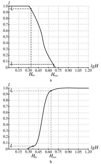
Fig. 1. Sensitometric curves of the elemental recording process: a - positive process; b - negative process
