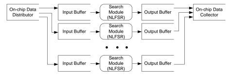
Fig. 3. Scalable implementation of brute force search task for FaaS
