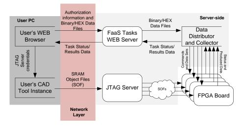
Fig. 2. Coarse-grained FaaS infrastructure
