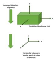
Figure 8: Plausibility of Acceleration Measurements
